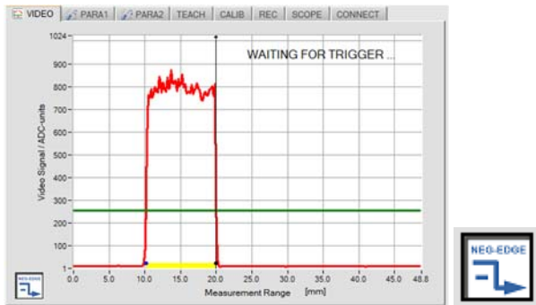
NEG-EDGE H/L-TRIGG at 20.0mm, Object: Gap Measurement G
